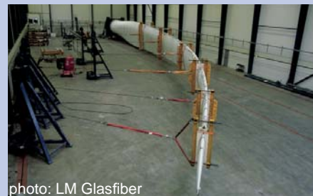
The world's largest testing station for blades is located at LM Glasfiber. Blades up to 80 m are tested at the station.
